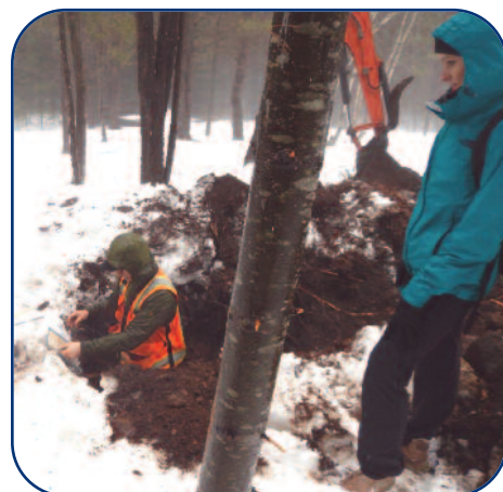
Above: Aaron Ziemann (in test pit) and Sarah Staab brave inclement weather to analyze a deep hole soil test pit to help property owner identify best location for onsite wastewater system.
