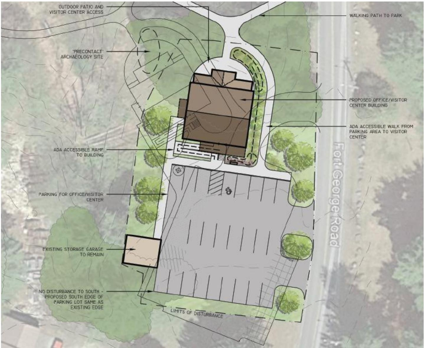
Figure 3. Proposed site plan layout for new facility. Previous proposed location shown outlined. “Pre-contact” archaeological fragments identified to the northwest of proposed building. Project will not impact this area.
