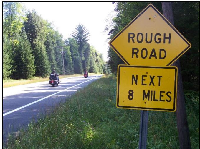
Frost and boulder heaves may be relieved by removing at least one of the three essential components. The water component may sometimes be eliminated by proper drainage. The soil or bedrock component is minimized by undercutting the susceptible material and replacing it with granular material. The freezing-temperature component is inherent to our climate and cannot be eliminated from the soil.
