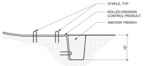
**SECTION TERMINAL ANCHOR TRENCH-DOWNSLOPE**
