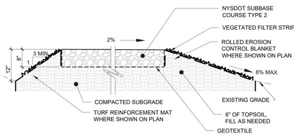
NOTE: TREATMENT OF THE SURFACE ADJACENT TO THE GRAVEL ROAD WILL VARY BASED ON ADJACENT GRADING. LOCATIONS OF THE OF TURF REINFORCEMENT MAT (TRM) AND EROSION CONTROL BLANKET (ECB) WILL BE IDENTIFIED ON THE GRADING PLAN.
