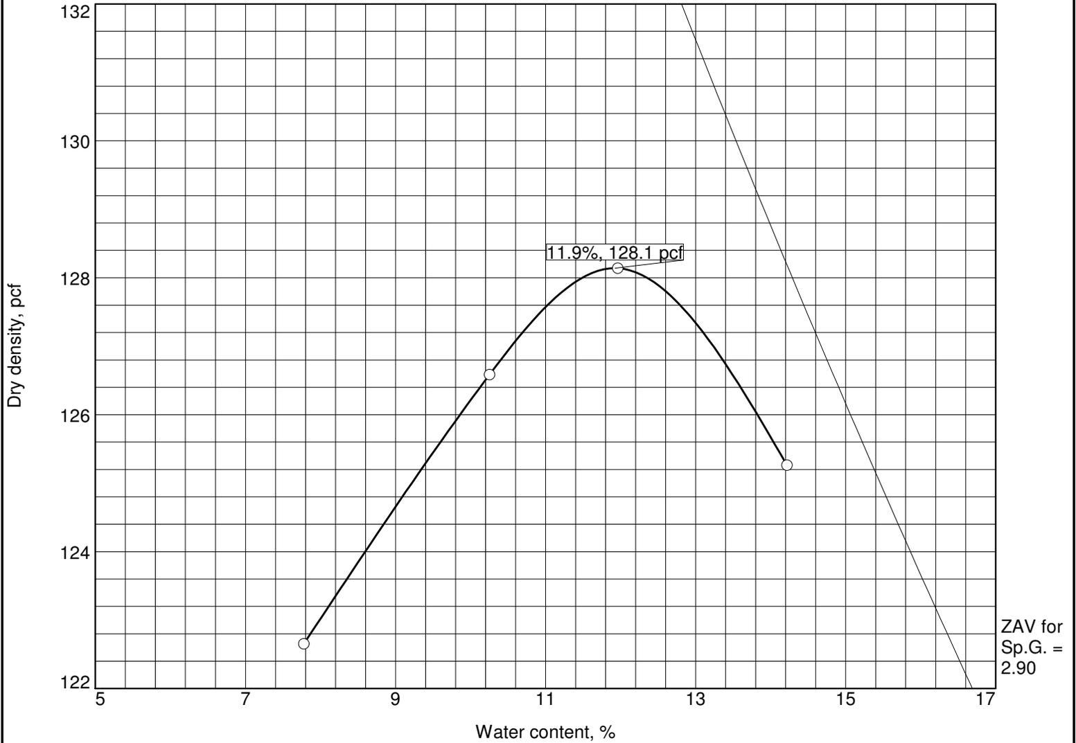
Test specification: ASTM D 1557-12 Method A Modified
