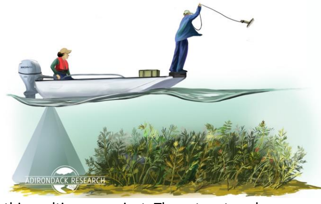
FIGURE 4. GRAPHIC DEMONSTRATING A RAKE TOSS USED FOR SAV SAMPLING
